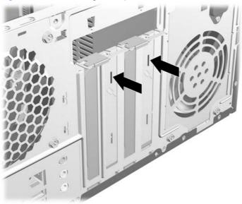
**b.** If you are removing a standard PCI card, hold the card at each end and carefully rock it back and forth until the connectors pull free from the socket. Be sure not to scrape the card against the other components.
